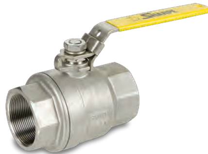
Full port 1000 WOG 316 Stainless Steel Locking device Blow-out proof stem Oval handle available
